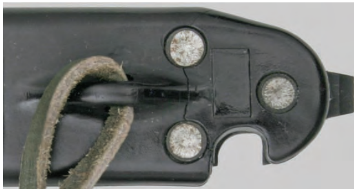
KCB-70 Scabbard with cracking at the stress point where the restraining lace attaches.
