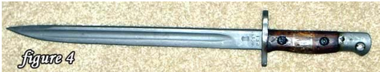
India Pattern No. 1 Mk. I** converted at Rifle Factory Ishapore.
