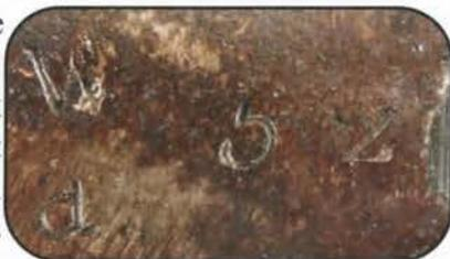
Figure 3: "W" over "a" and "52" marking on Type I fencing socket.
